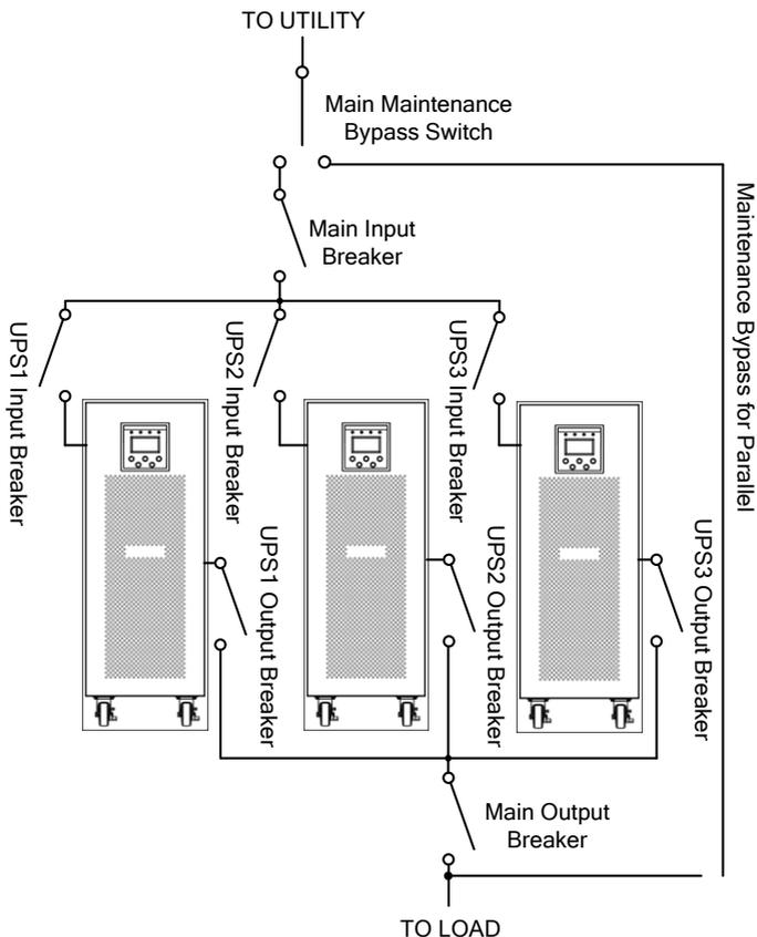
Fig.6-3 Parallel installation diagram
