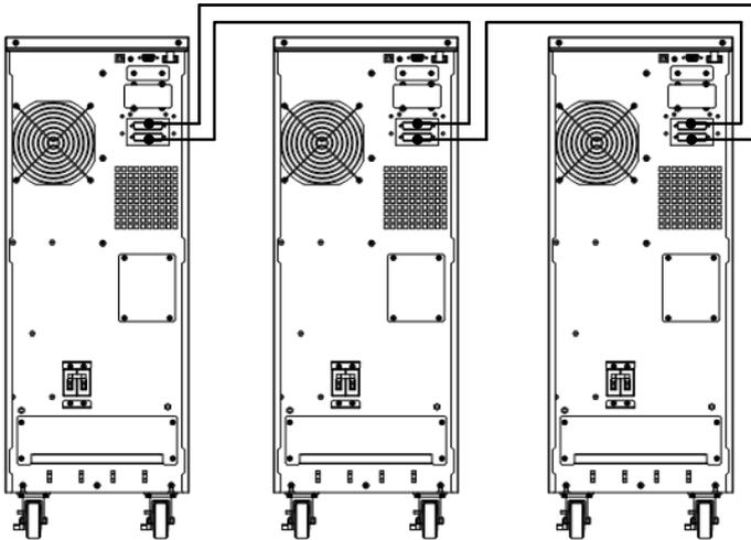
Fig.6-1 Parallel cable connect diagram
