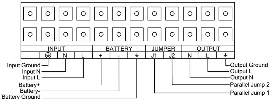
Fig.4-2 Input and output Terminal Block wiring diagram
