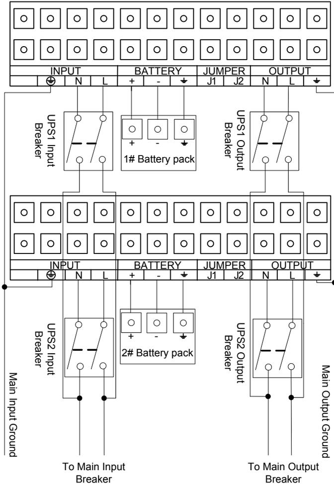
Fig.6-2 Input and output Terminal Block wiring diagram
