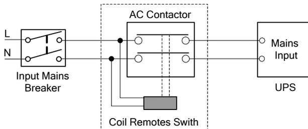
Fig.4-1 Typical external isolating device installation
